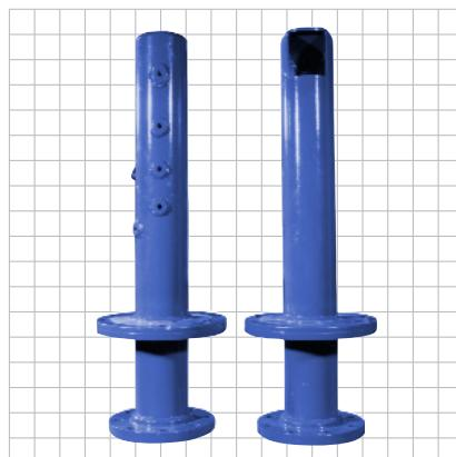
The enclosure contains a flow-through Cell sampler which discharges 1cc samples directly into a sample receiver. The short distance travelled by the sample minimises the risk of cross-contamination between batches.
